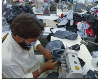
Photo of non-conformity NC workers on over lock machines were not using eye guards as PEEs.jpg
